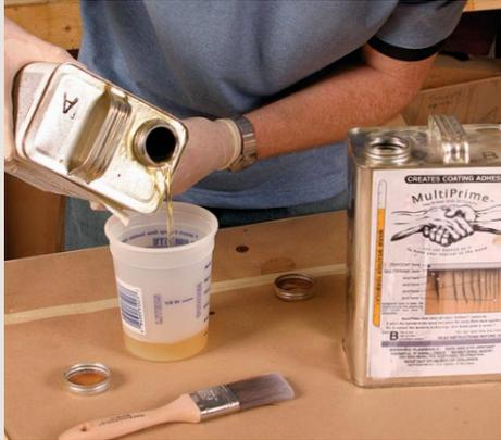
**Mix the primer.** The epoxy comes in two parts that are blended in equal measure.
